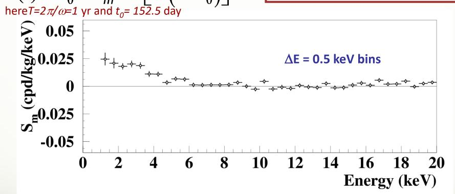
A clear modulation is present in the (1-6) keV energy interval, while  $S_m$  values compatible with zero are present just above
